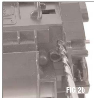
**Note:** If the drill does not push the pin out of the cartridge, use the HP1200 pin removal tool to push the pins out of the cartridge.
