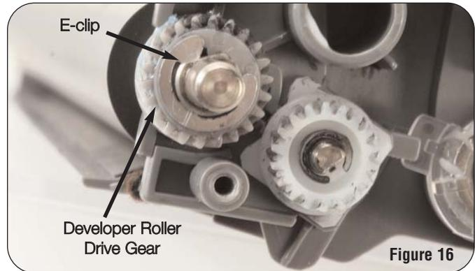
4. Replace the gears (1-3) and then the developer roller contact as shown in Figure 17.
