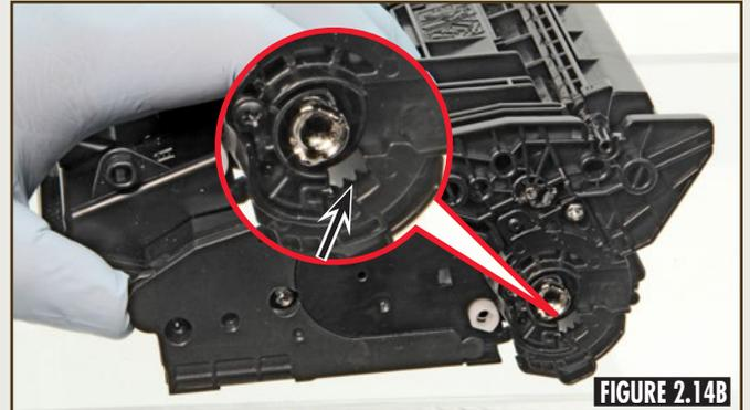
Press the lever on the back side of the SCC drive side hopper end plate to ensure the OPC drive gear protrudes and retracts, as shown in Figures 2.14A and 2.14B.
