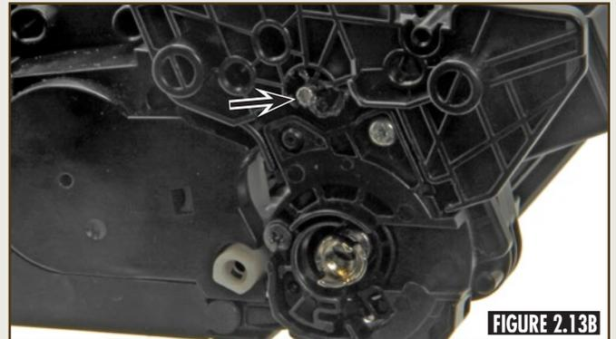
Install the OEM cartridge pins on both sides of the cartridge, as shown in Figures 2.13A and 2.13B.
