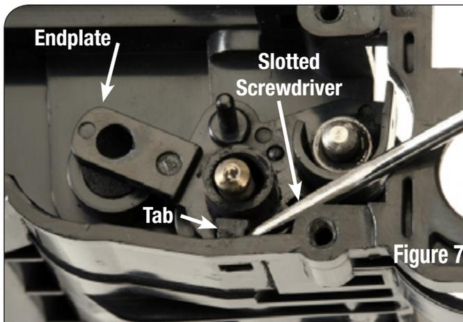
3. Slide the endplate off the shafts.
