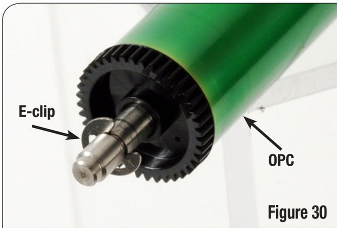
7. Apply a small amount of conductive lubricant on the OPC axle between the e-clip and the spur gear (Figure 31).
