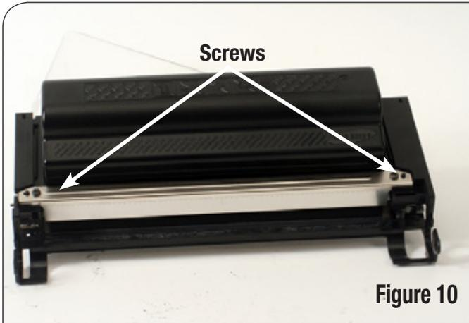
8. Inspect the doctor blade and hopper to ensure all foams and felts are in good condition. Replace as necessary.
