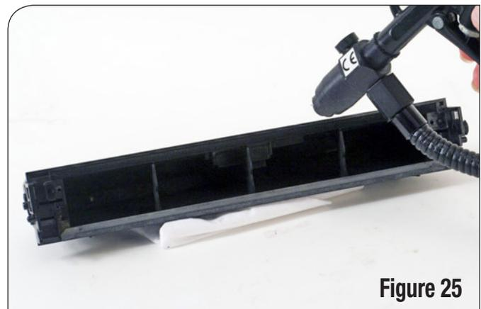
8. Inspect the recovery blade for damage. Replace if necessary.
