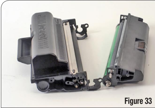
2. Press the two sections together until the locking tab on the sides snap into place (Figure 34a and 34b).
