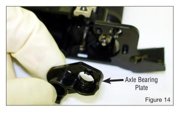
6. With the axle bearing plate removed, the developer roller can be removed. Lift the contact side (non-geared side) of the developer roller out and away from the hopper section. See Figure 15 & 16.
