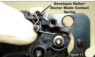
3. Use a slotted screwdriver to release the long leg of the contact spring from the developer roller. Then remove the spring from the hopper as shown in Figure 12.
