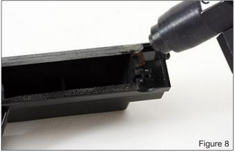
3. Before installing a new wiper blade, be sure to dip the working edge of the wiper blade in toner for lubrication. Install the new wiper using the two screws that were removed as shown in Figure 9.
