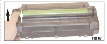
**3.** Install the Drum Shutter as shown. FIG 68 shows the position of the helical side shutter arm and FIG 69 shows the position of the spur side shutter arm. Be sure that the springs are placed in the proper position, see figures below.
