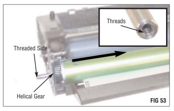
16. Place the Developer Roller drive gear on the cartridge as shown (FIG 54).
